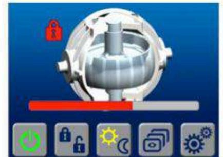
To start, press the POWER ON/OFF. A RED PROGRESS BAR will appear. When the GYRO reaches operating speed the PROGRESS BAR will turn GREEN. The GYRO is available for stabilization.
