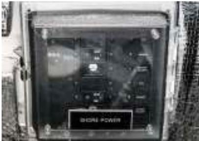
SHORE POWER BREAKER BOX located on starboard hull over the GENERATOR. If no AC power showing on Panel, check to be sure the BREAKERS aren't tripped.
