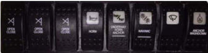
**Windshield Actuators** Three switches operate the electric synchronous actuators that open the windshields (option).
