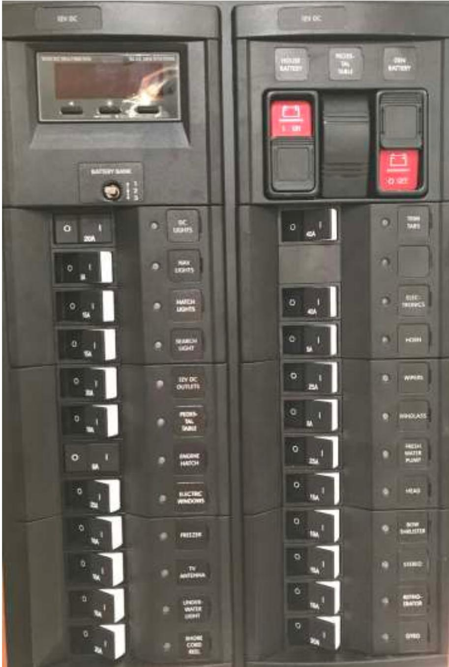
The TOGGLE switch below the digital display on the 12V DC panel shows volts or amps for the HOUSE BATTERIES in position 1 and the GENERATOR BATTERY in position 2. Position 3 is not connected.
